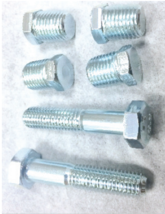
Figure 13 – Pavco SmartZinc Premier barrel plated at 2.2 A/dm 2 , 13 µm on bolt heads in 15 min, with no stardusting.
