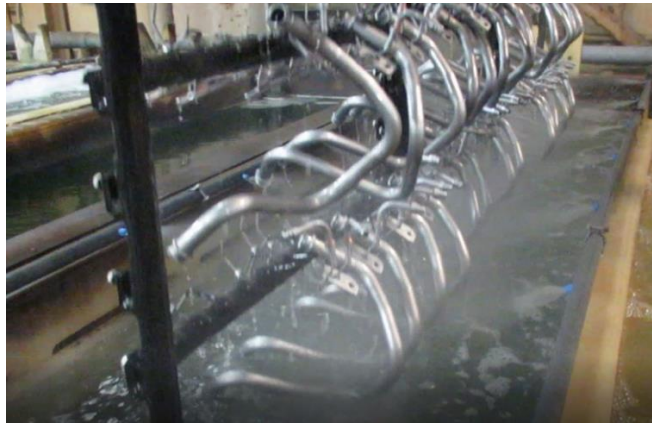
Figure H-6. Spray Rinse on Tank 111
