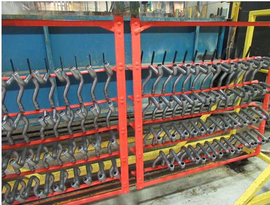
Figure H-10. Racks with New Plastisol Coatings
