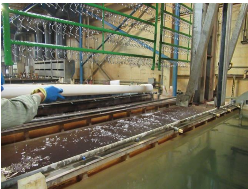
Figure H-5. Sampling Drainage After Rack Removed From Tank
