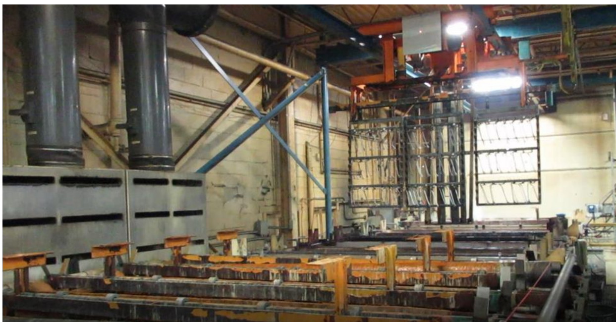
Figure H-1. Automated Zinc/Nickel Rack Plating Line
