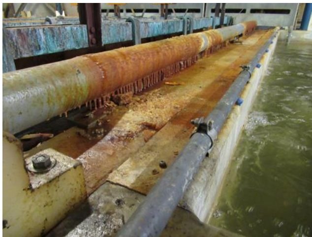
Figure H-11. Pictures of Zn/Ni Tank Before and After Installation of Drip Board
