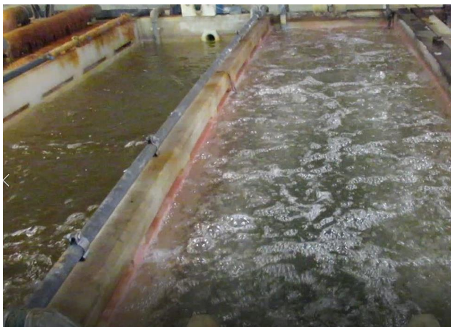
Figure H-3. Visual Comparison of Tanks with Poor (left) and Good (right) Air Agitation
