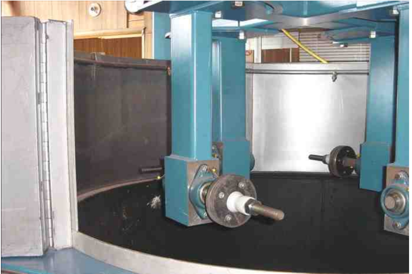
Figure 8. Empty Loading Fixtures
