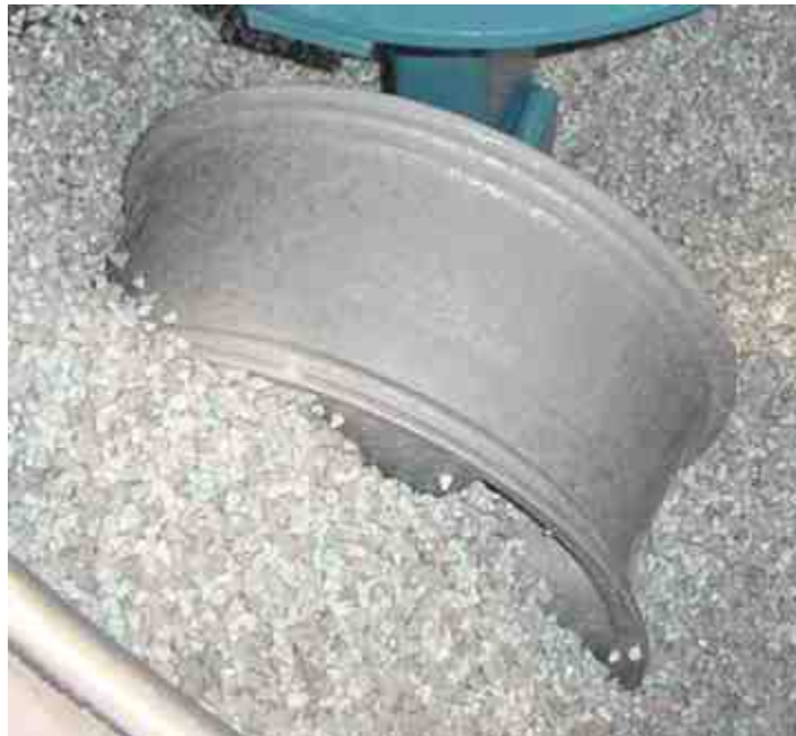
Figure 1. Wheel # 1 being pushed face first through media.
