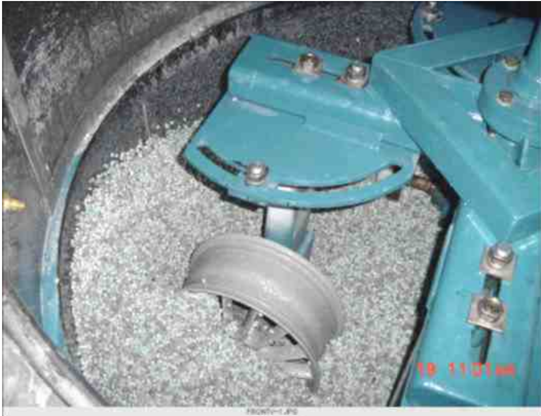
Figure 3. Wheel # 2 being pushed face first through media.
