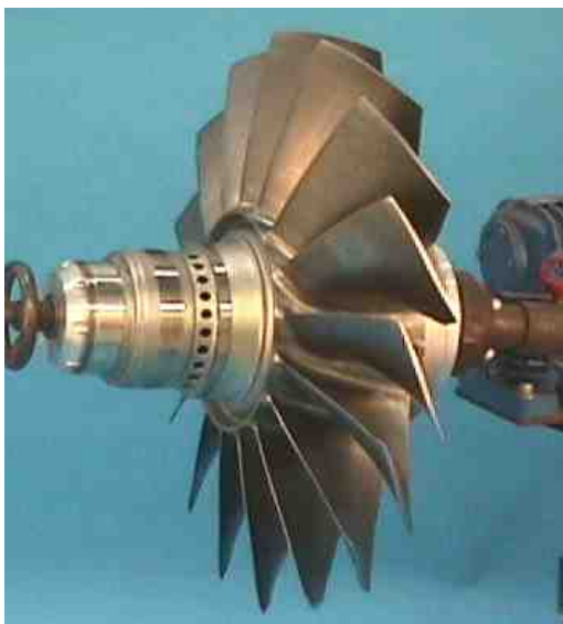
Figure 8.5 – Blisk finished by ECM
