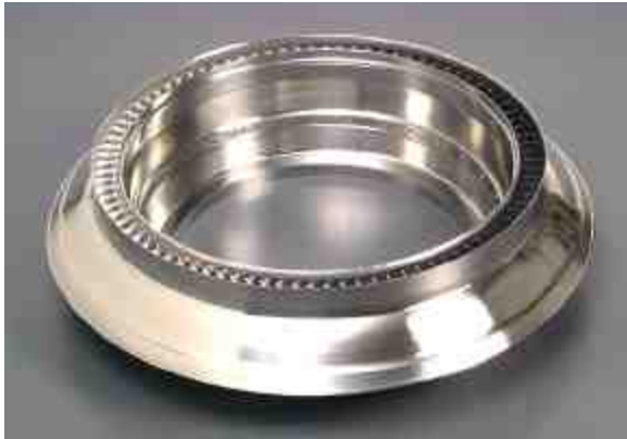
Figure 8.7 – OGV – vanes cut by ECM
