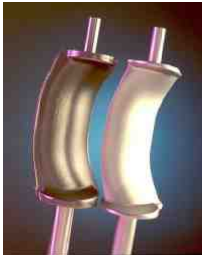
Figure 8.10 ECM Vane from a forging
