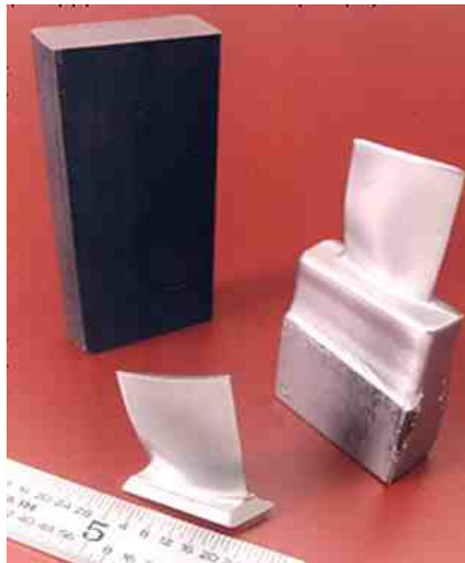
Figure 8.9 – ECM Blade from bar stock
