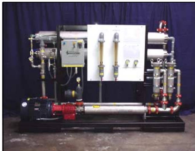
Figure 3. Perfection Plating's RO System
