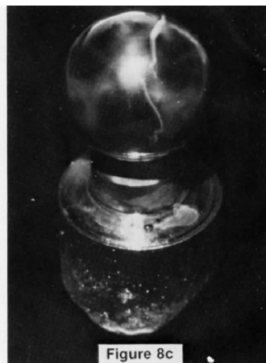
Figure 8 - Optical micrographs of a single crystal sphere subjected to a 1-min zincate immersion followed by a dip in 50% nitric acid to strip off the zinc (a) the (100) plane, (b) the (110) plane and (c) the (111) plane.
