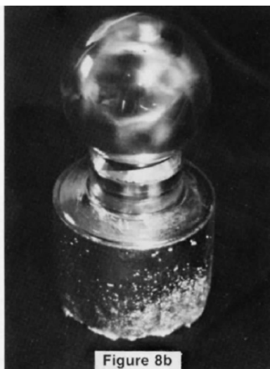
Figure 8 - Optical micrographs of a single crystal sphere subjected to a 1-min zincate immersion followed by a dip in 50% nitric acid to strip off the zinc (a) the (100) plane, (b) the (110) plane and (c) the (111) plane.
