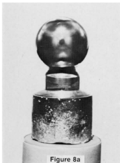
Figure 8 - Optical micrographs of a single crystal sphere subjected to a 1-min zincate immersion followed by a dip in 50% nitric acid to strip off the zinc (a) the (100) plane, (b) the (110) plane and (c) the (111) plane.
