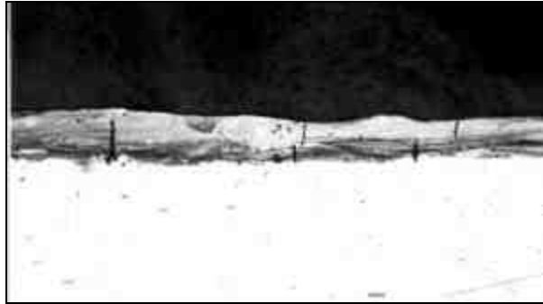
Fig. 8 – ESD Chromium Carbide showing optimum stress-relief crack pattern.
