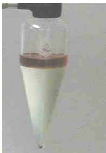
Fig.1. Three phases sample after percentrifugation using cyclohexane as the extracting solvent.
