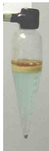
Fig. 2. Example of a well-separated sample showing four distinct phases.
