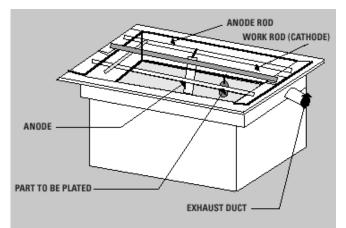
Figure 2: Main components of an electroplating tank. Air is exhausted with a perimeter slot exhaust.
