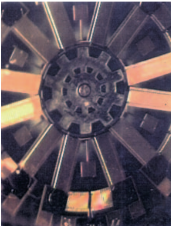
Fig. 12—The assembled motor with a 6-mm diameter rotor in place, surrounded by 6 horseshoe magnets.
