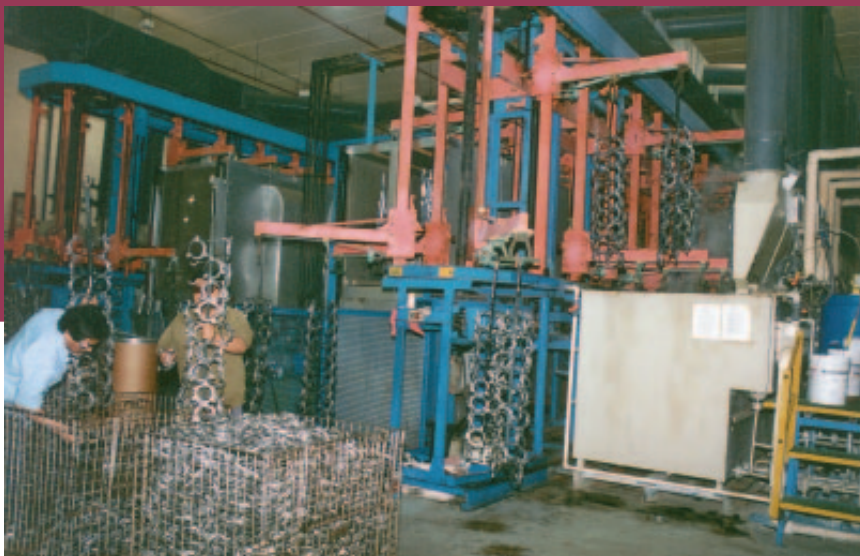
The ultra-modern plating facility offers just-in-time delivery service that appeals to its appliance and automotive industry customers. Workers are unranking neck rings for home garbage disposal units that have just been finished on one of the shop's four return-type automatic machines.
