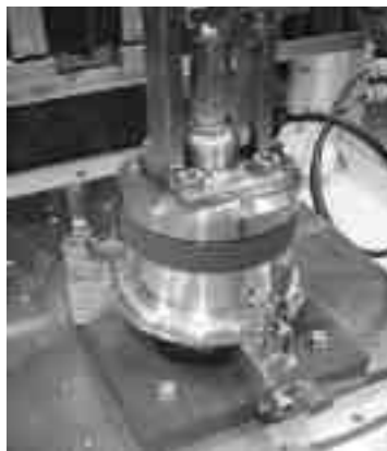
Fig. 8—Fixturing for aluminum-alloy wheel finishing.
