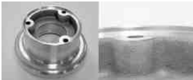
Fig. 5—Aluminum-alloy wheel edge burrs to be deburred.
