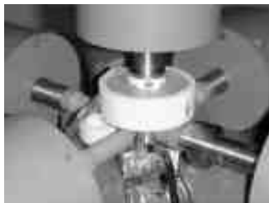
Fig. 7—Fixturing for stainless steel valve finishing.
