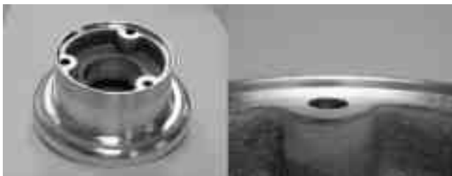
Fig. 13—Edge appearance of aluminum alloy wheel after electrically-mediated finishing.
