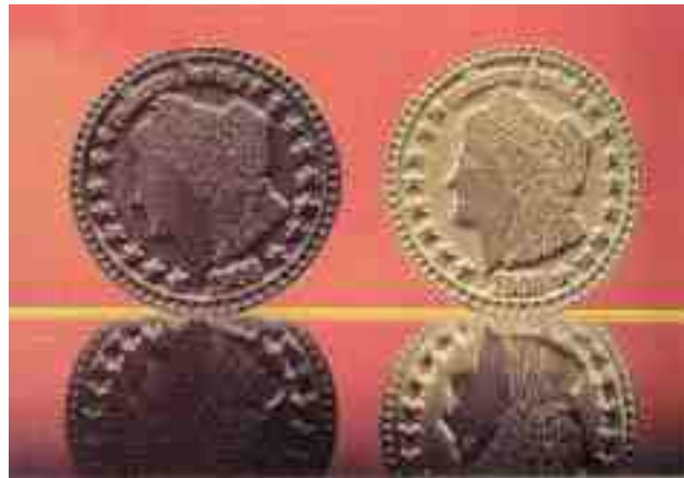
Fig. 3—Commemorative coins with coating produced by hot alkaline blackening.
