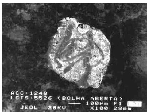
Figure 5—A blister after removal of the zinc coating. The scratches are due to the tool used. Magnification: (Left) 100X; (Right) 700X. No etching.
