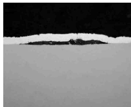
Figure 3—Cross-sections of blistered parts showing separation at the steel/zinc interface. Magnification: 1000X. No etching.
