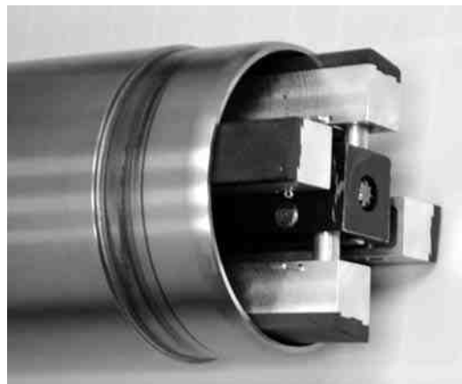
Setup for internal honing operation using FriCSo polymer inserts.
