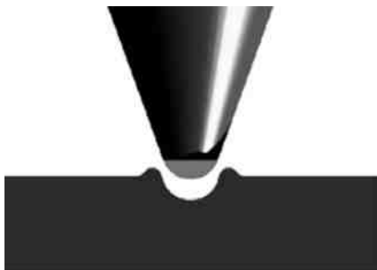
Schematic cross-section of the grooving process, showing the ridges formed by plastic deformation.
