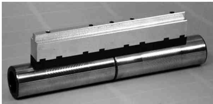
Typical external diameter lapping fixture with attached FriCSo polymer insert (the darker element in contact with piston pin). Note the grooved surface texture on left half of the piston pin.
