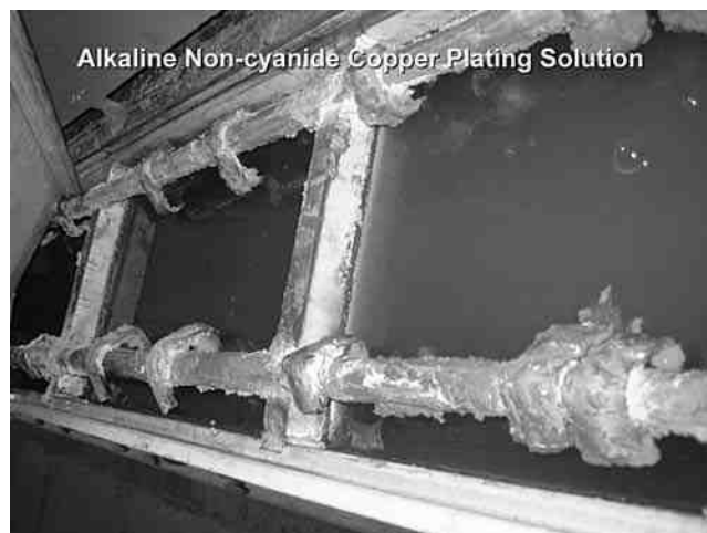
Photo 2—Tank with copper plating solution showing limited free-board and accumulated salts.
