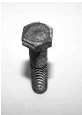
Unretouched photo illustrating the result obtained by placing a drop of diphenylcarbazide solution on the top of a trivalent passivated fastener and placing it in the salt spray cabinet for 24 hours. [Original color photo shows a purple color in the slightly darker shading within the center of the head (about half the diameter) - Ed.]
