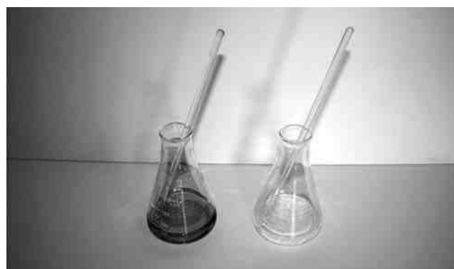
Erlenmeyer flask showing the typical red-violet color of the complex formed between hexavalent chromium and 1,5-diphenylcarbazide. The sample on the left was prepared by diluting and acidifying the condensate from a commercial trivalent passivate obtained from the ASTM B-117 Salt Spray Test and treating the solution with 1,5-diphenylcarbazide at a reduced pH. The Erlenmeyer flask on the right illustrates the result obtained from a control sample that was unpassivated.
