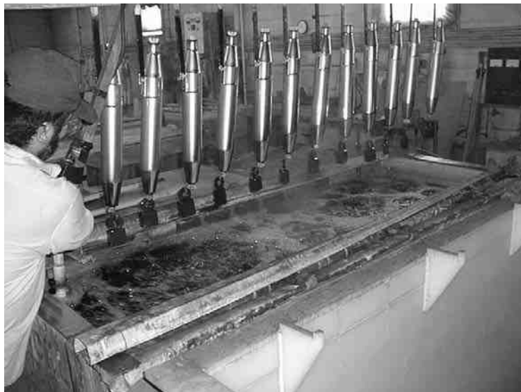
Figure 3—Racking of hollow parts showing plugged ends and weights.
