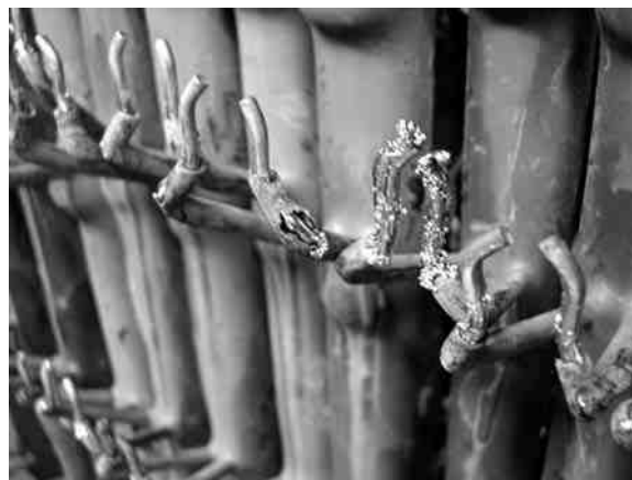
Figure 1—Metal buildup and split coating on rack needing extensive maintenance.
