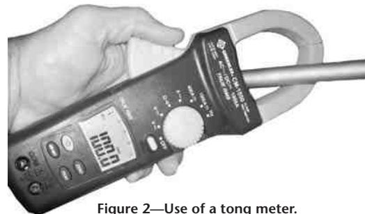
Figure 2—Use of a tong meter.
