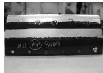
Figure 4—Sol-gel rivet finish.
