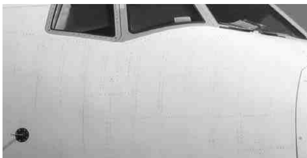
Figure 9—Rivet rash on a Boeing 777 painted prior to sol-gel rivet conversion after 18 months in-service.
