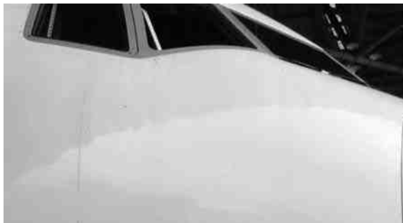
Figure 10—Minimal rivet rash on a Boeing 777 painted after sol-gel rivet conversion after 14 months in-service.
