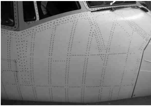
Figure 1—Severe “rivet rash” by flight deck window.
