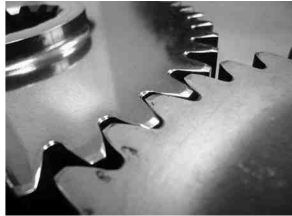
Figure 10—Superfinished gear (L) and as ground (R).
