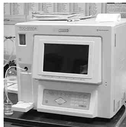
Figure 2—Shimadzu 5050A TOC analyzer
