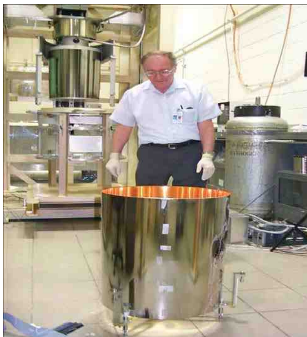
Figure 9—A 0.25-mm thick NiCoP electroformed x-ray mirror with a gold inner surface.
