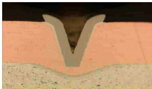
Figure 6—NiP electroplated in a 0.25-mm drilled taper hole.
