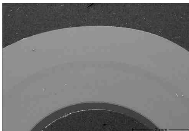
Figure 5—A 0.3-cm (3-mm) thick NiCoP electrodeposit: Hardness ( HV_{0.1} ) - 550, 560, 580, 540, 580, 590, 580 (inside to outside).
