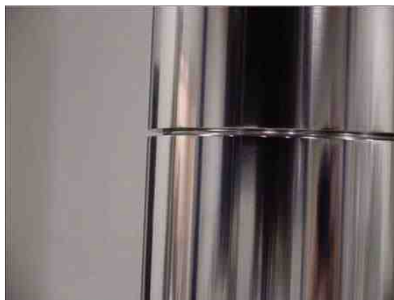
Figure 8—An as-plated 0.25-mm thick NiP electrodeposit on a 15-cm diameter mandrel.
