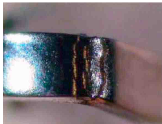
Figure 12—Cracks in the nickel layer, with excellent bonding of the Pd-Ni after the bend test.
