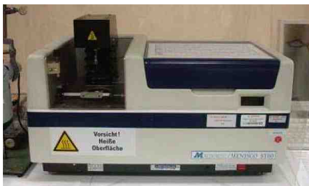
Figure 8—Wetting balance equipment used to measure solderability of lead-free solders (wrt ZCT).
