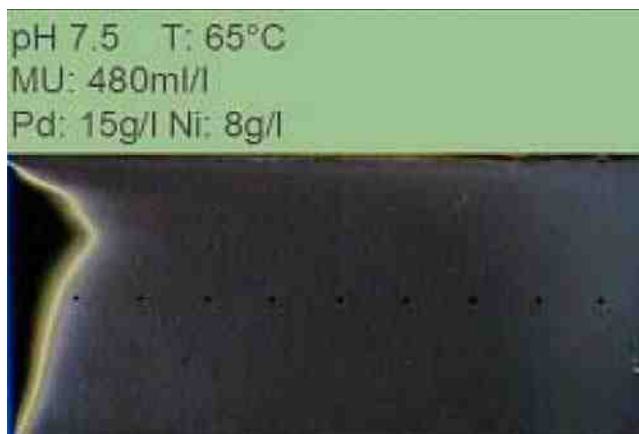
Figure 2—Typical bright and homogeneous deposit of electrodeposited Pd-Ni alloy as shown by Hull cell.
