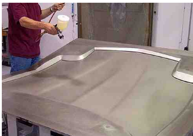
Figure 1—Invar tool for Corvette carbon fiber hood outer production.
