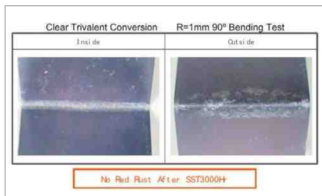
Figure 7—Bend test results after 3000 hr neutral salt spray (NSS).
