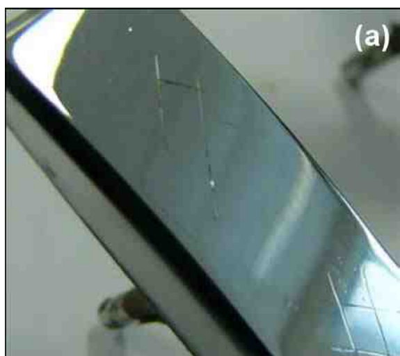
Figure 3 —CASS test results for plated plastic without micro-porous nickel plating after six cycles - with scratches prior to test: (a) crack-free chromium plating (CF Cr); (b) conventional hexavalent chromium plating (HV Cr).
