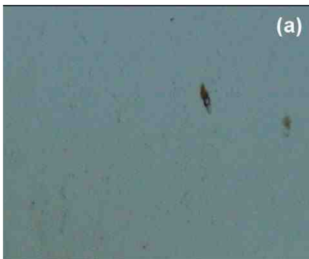
Figure 5 —CASS test results for tri-nickel plating on iron after 4.5 cycles: (a) crack-free chromium plating (CF Cr); (b) conventional hexavalent chromium plating (HV Cr).
