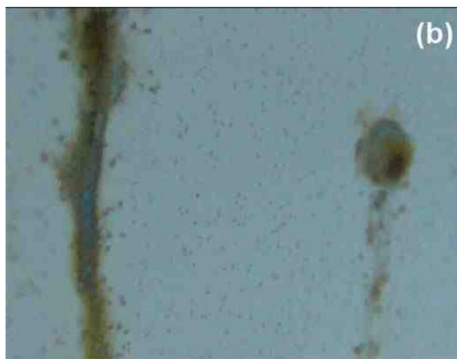
Figure 5 —CASS test results for tri-nickel plating on iron after 4.5 cycles: (a) crack-free chromium plating (CF Cr); (b) conventional hexavalent chromium plating (HV Cr).
