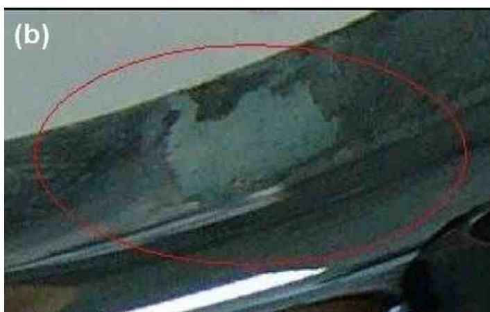
Figure 4 —Calcium chloride + kaolin corrosion test results for plated plastic with micro-porous nickel plating after one week: (a) crack-free chromium plating (CF Cr); (b) conventional hexavalent chromium plating (HV Cr).
