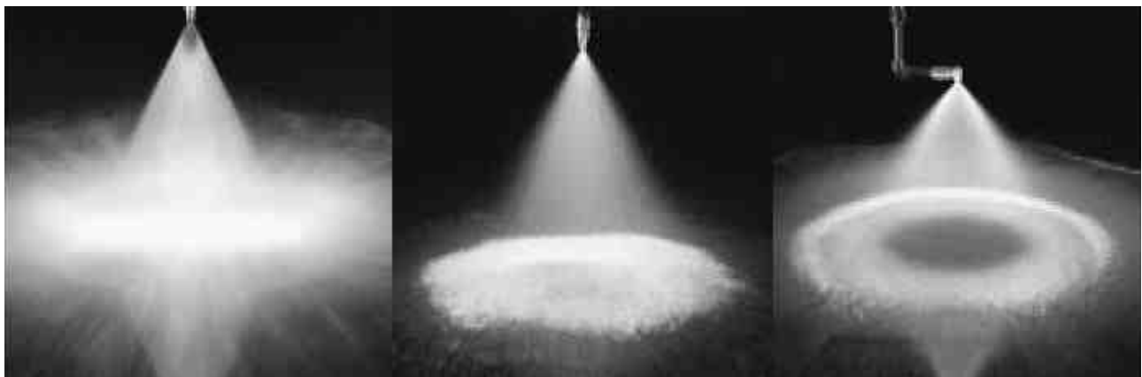
Figure 8 —Flat, full cone and hollow cone spray nozzle pattern (Photos Courtesy of Spraying Systems Co., Farmington Hills, MI).
