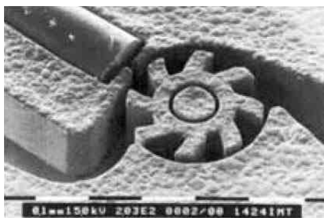
Figure 22 —Electroformed nickel micro-turbine made by the LIGA process.
