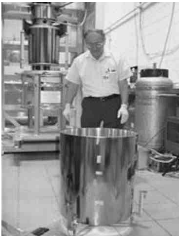
Figure 15 —Ni-Co-P alloy large x-ray mirror test cylinder (Photo courtesy of University of Alabama, Huntsville, AL).
