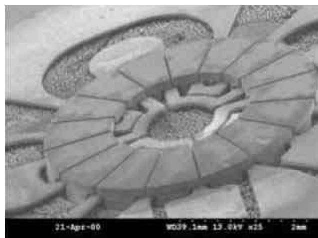
Figure 20 —Electroplated Ni-Fe alloy core and copper windings in a planar induction motor.
