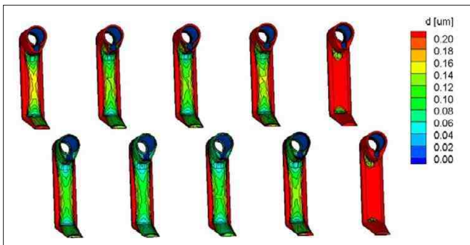
Figure 9—Chromium layer thickness distribution over lower parts on rack, Case 2.
