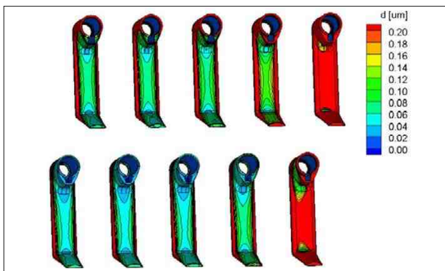
Figure 7 —Chromium layer thickness distribution over lower parts on rack, Case 1.
