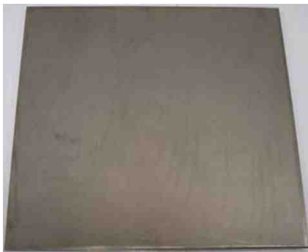
Figure 5 —15 cm × 15 cm × 0.3 cm Nb foil, 99.9% pure.
