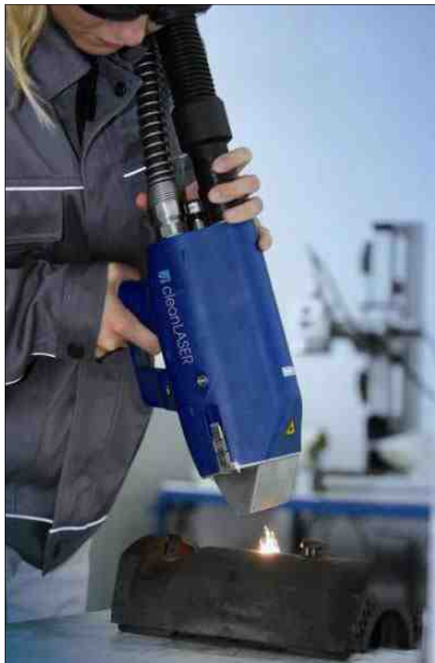
Figure 5—Manual laser cleaning with a 300 W laser.
