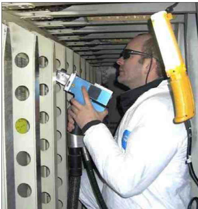
Figure 4—Paint removal in B-52 center tank.
