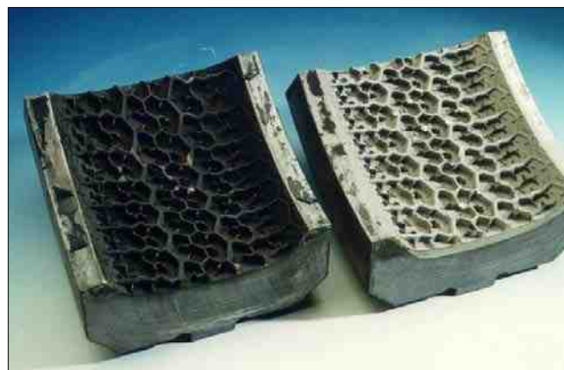
Figure 6—Laser-cleaned tire mold.
