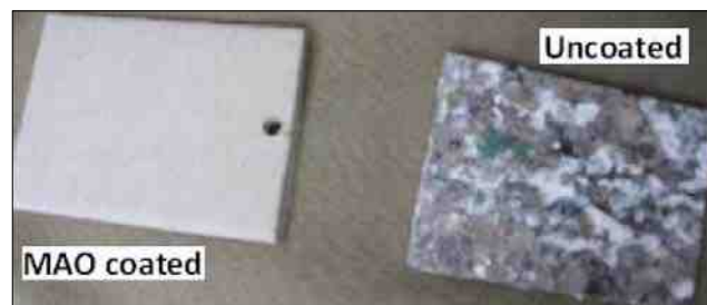
Figure 7 —Salt spray tested MAO-coated and uncoated specimens.
