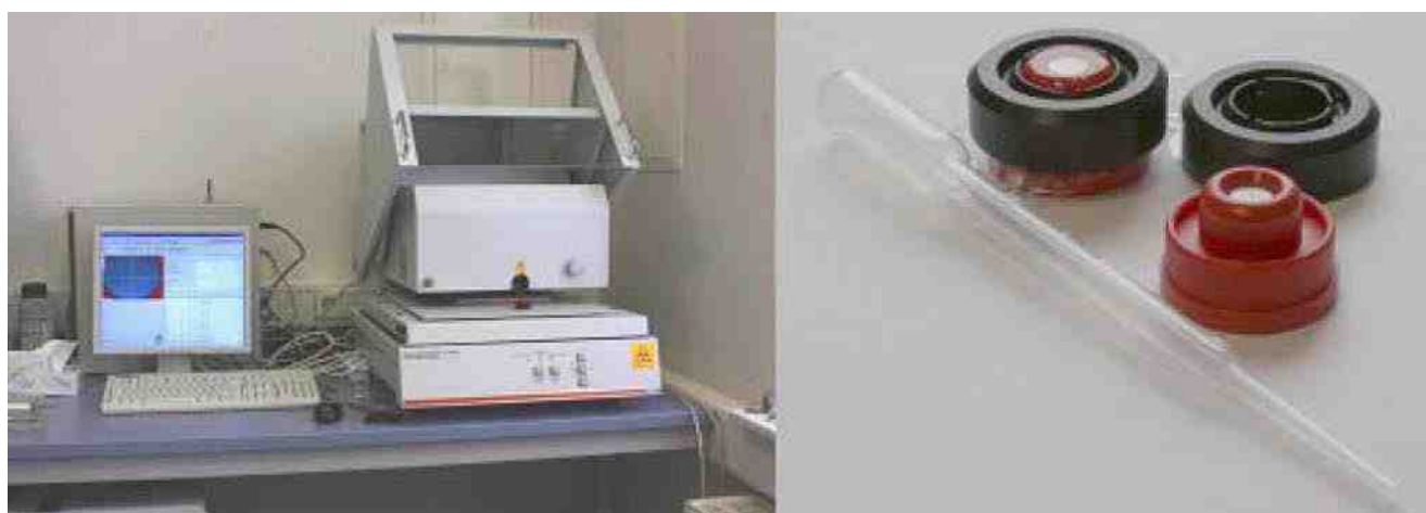
Figure 6—XRF equipment and test cell for XRF analysis of liquids.
