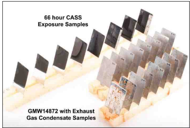
Figure 8 —All sets after CASS and GMW-14872 cyclic corrosion testing.
