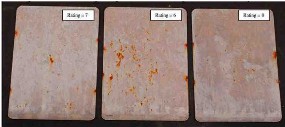
Figure 7 —Panels showing ratings 6, 7 and 8 after 25 cycles of GMW-14872 exposure.
