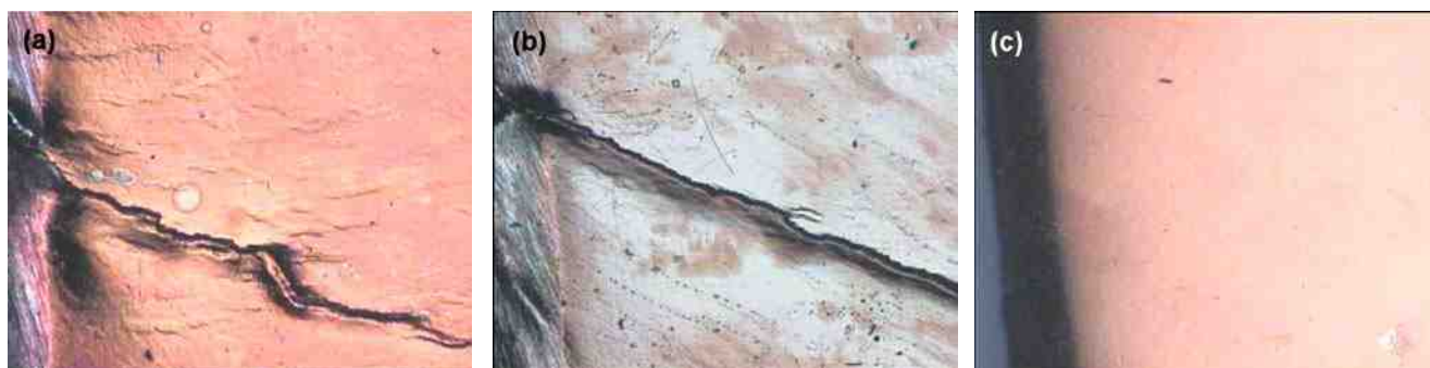
Figure 4 —Plated copper ABS (P2MC) test plaques at the shear cut line (50×): (a) standard 400 g/L Cr(VI); (b) standard 1000 g/L Cr(VI); (c) direct process.
