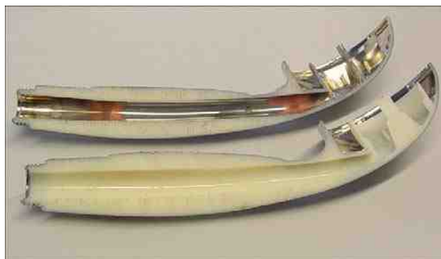
Figure 5 —Lengthwise cross-section of two hand shower parts processed in the standard process (top) and the new direct metallizing process (bottom).
