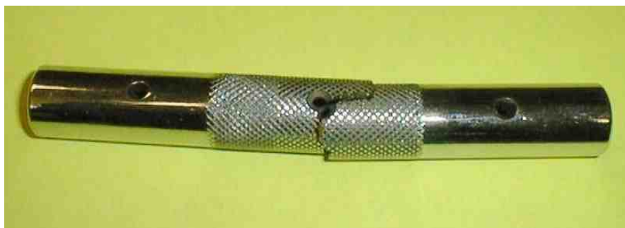
Figure 1 - Failure of marine turnbuckle resulting from stress corrosion cracking.
