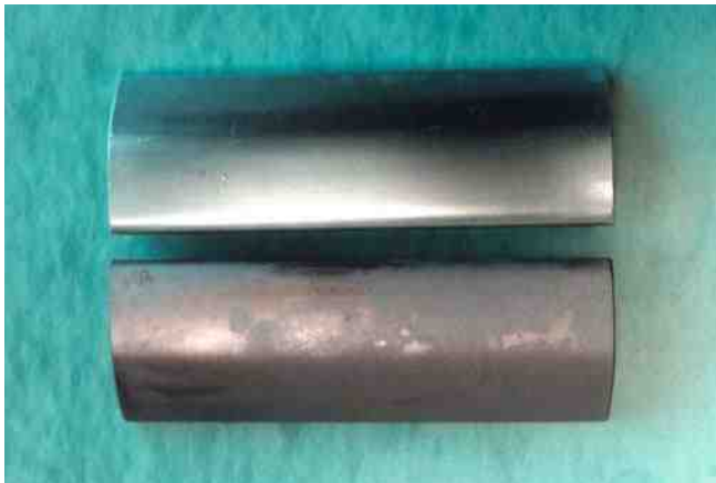
Figure 1 - Beryllium/aluminum alloy before and after (top) being plated with electroless nickel.
