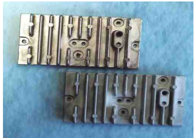
Figure 3 - Plated cast aluminum alloy before (top) and after being plated with electroless nickel.
