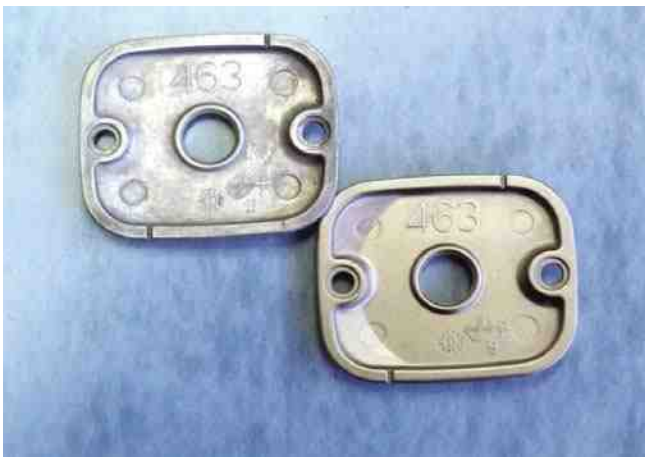
Figure 2 - Plated magnesium before (top) and after being plated with electroless nickel.
