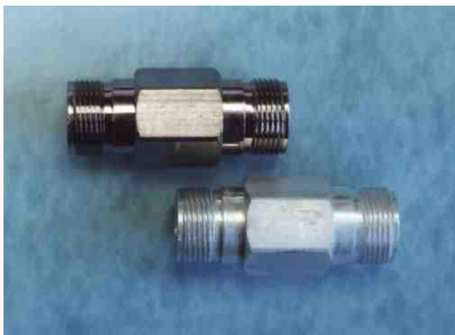
Figure 4 - 6061 extruded aluminum alloy before (top) and after plating with electroless nickel.
