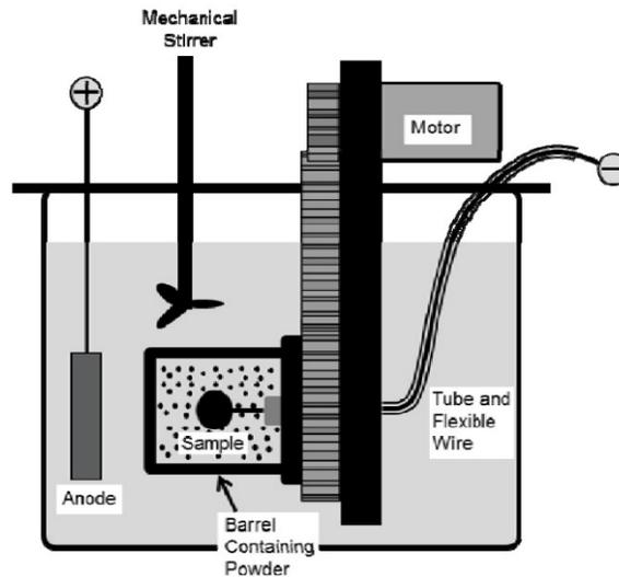
Figure 1 - Schematic of the barrel system.
