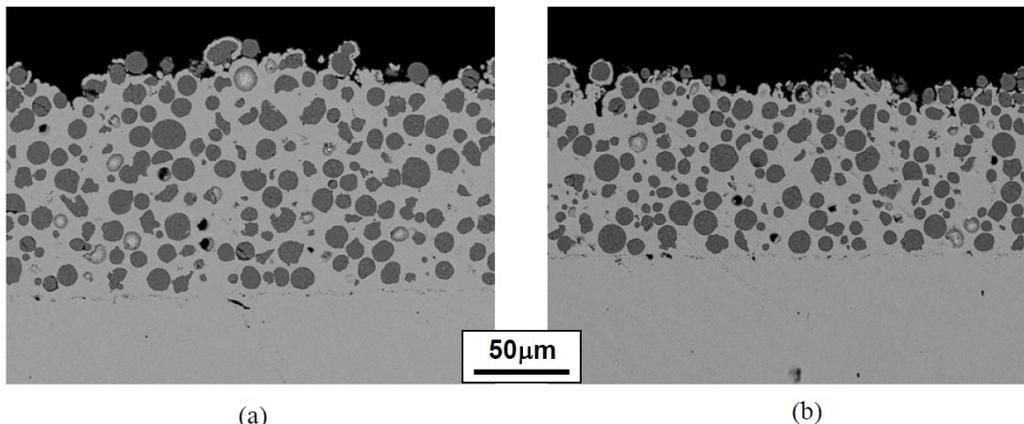
Figure 2 - SEM cross-sectional images of the Ni-CrAlY coatings fabricated with the atomized CrAlY powders at different current densities: (a) 10 mA/cm<sup>2</sup>; (b) 60 mA/cm<sup>2</sup>.
