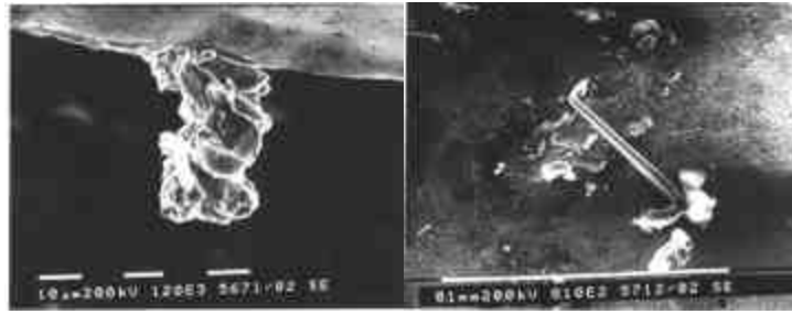
Figure 6. Typical Tin Whiskers in Tin Deposits
