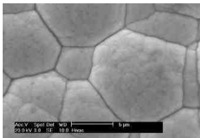
Fig. 8- Surface topography of 40 \mu\text{m} thick Co-W.
