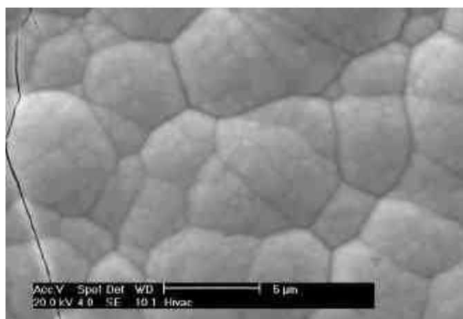
Fig. 7-Surface topography of 20 \mu\text{m} thick Co-W.
