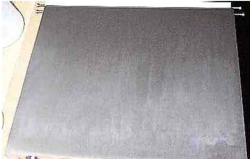
Patterned EN deposit due to pretreatment issues
