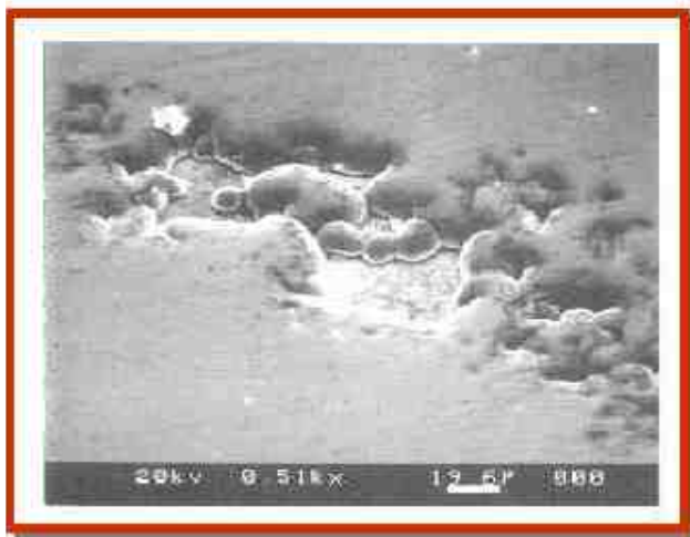
Void in EN coating due to improper pretreatment
