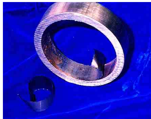
Adhesion failure ID surface
