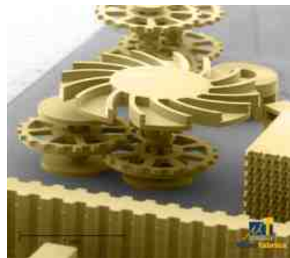
Fig. 14. Fluid-driven impeller with reduction gearing (1 mm tall). 62
