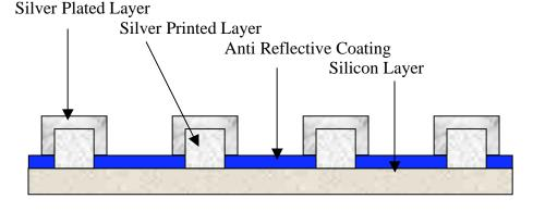
In this new method the thinner, narrow, screen printed silver layer fires through the anti reflective layer and is then over plated with 10 microns of silver. This total combination then becomes the total silver conductor layer
