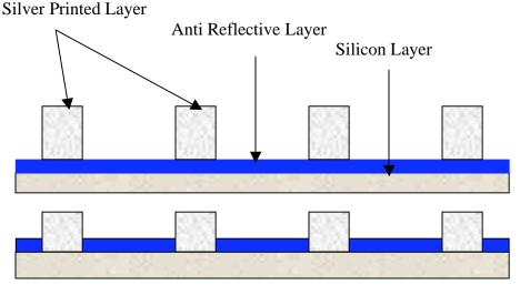
In this traditional method the screen printed silver layer fires through the anti reflective layer and becomes the total silver conductor layer
