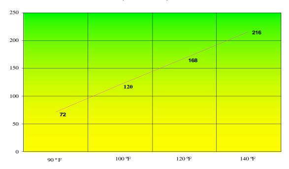
Red rust results with 0.0003" of zinc are hours to red rust failure.
