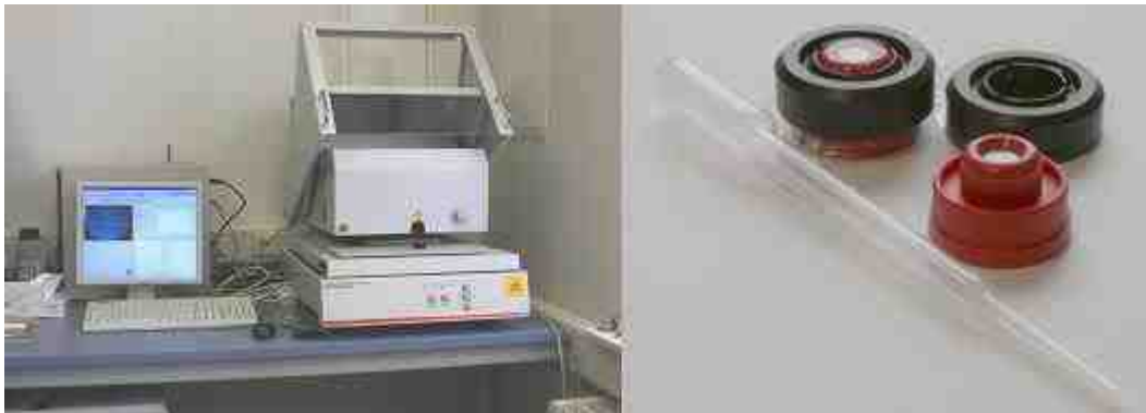
Fig 6: XRF equipment and test cell for XRF analysis on liquids.
