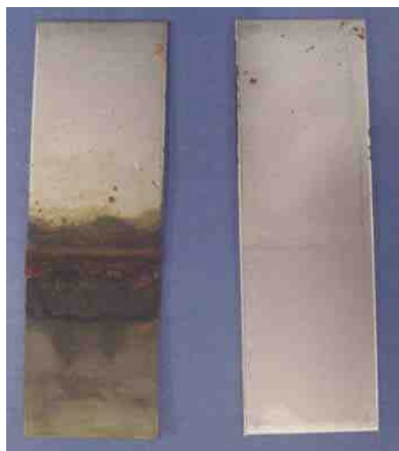
Figure 2: Corrosion performance of 1010 steel panels partially immersed in DI water for nine months with the different inhibitors at 0.10% active level: a) didecyldimethylammonium chloride (DDAC) and b) didecyldimethylammonium bicarbonate/carbonate (DDABC).
