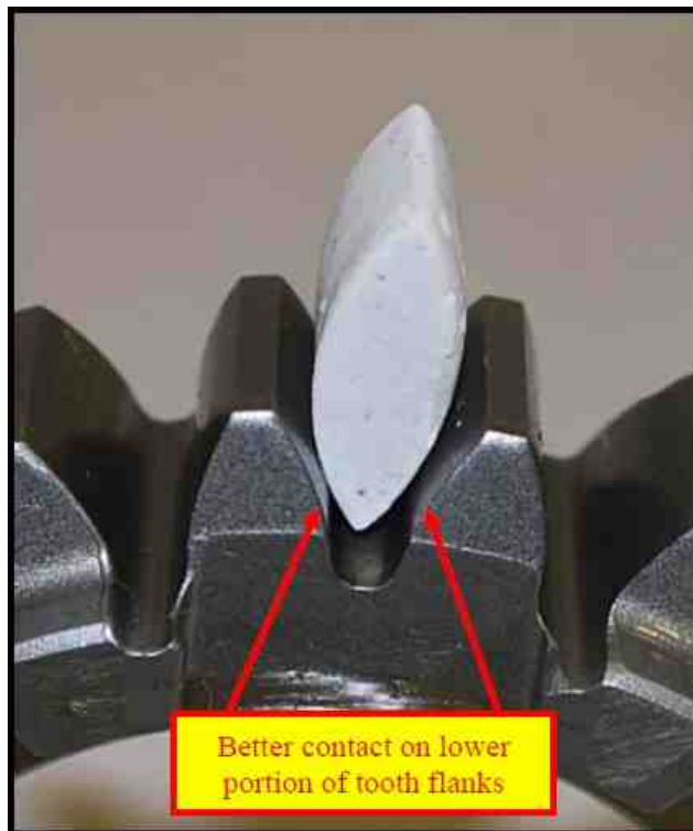
Figure 15 - An ellipse-shaped media is a better choice than a cylinder for more efficient contact on the gear tooth flanks.
