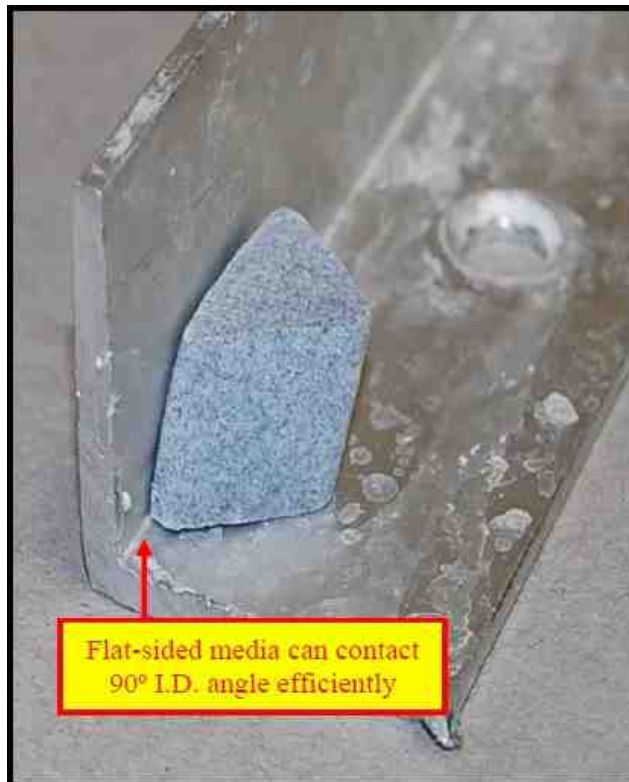
Figure 14 - An angle cut triangle, the flat faces of which ensure more efficient contact in the 90° I.D. corner.
