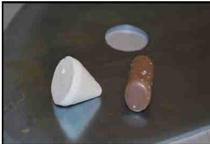
Figure 6 - Linear contact pattern No. 1: flat work piece and linear, tangential, media contact.
