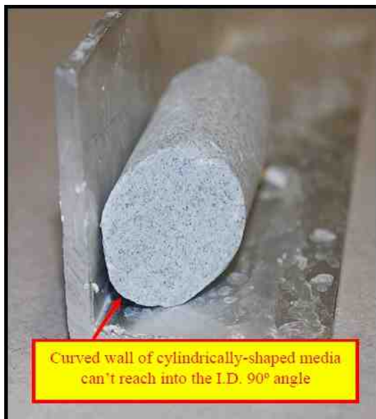
Figure 12 - A cylindrical piece of media that is being used to deburr an I.D. 90° angle. The curved side of the cylinder prevents its contact in the I.D. corner.
