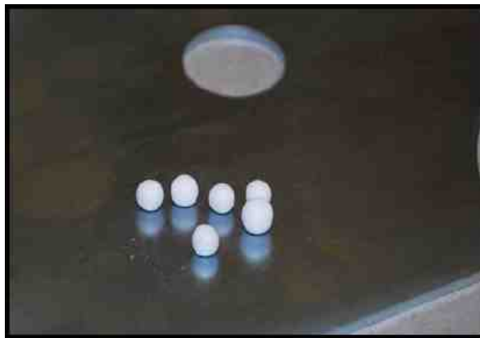
Figure 9 - A point contact pattern which occurs when a sphere contacts a flat face. In this example, the work piece is flat and the vibrate processing media is spherical.
