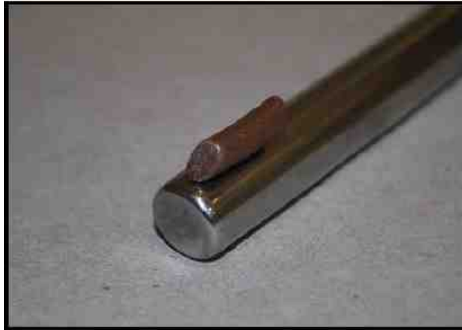
Figure 8 - Linear contact pattern No. 3: curved part contacted by curved media.
