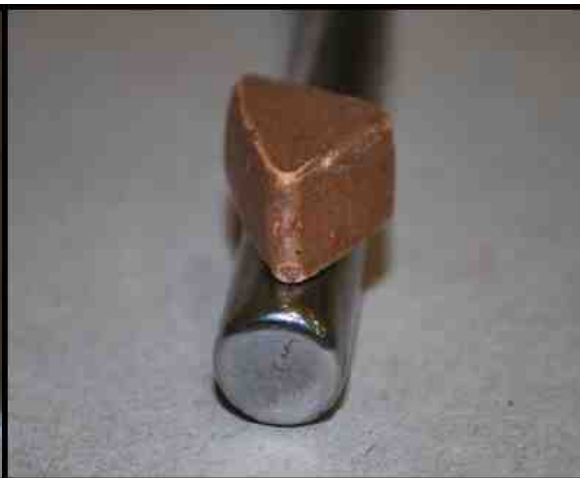
Figure 7 - Linear contact pattern No. 2: curved part contacted by a flat media face.
