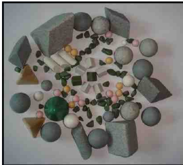
Figure 2 - An assortment of ceramic and plastic media in a variety of sizes and shapes.
