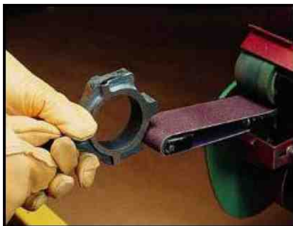
Figure 1 - An automotive connecting rod being hand polished with a polishing belt.
