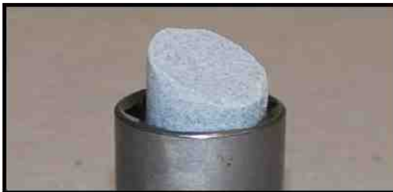
Figure 10 - A cylindrical work piece containing lodged, cylindrically-shaped media.
