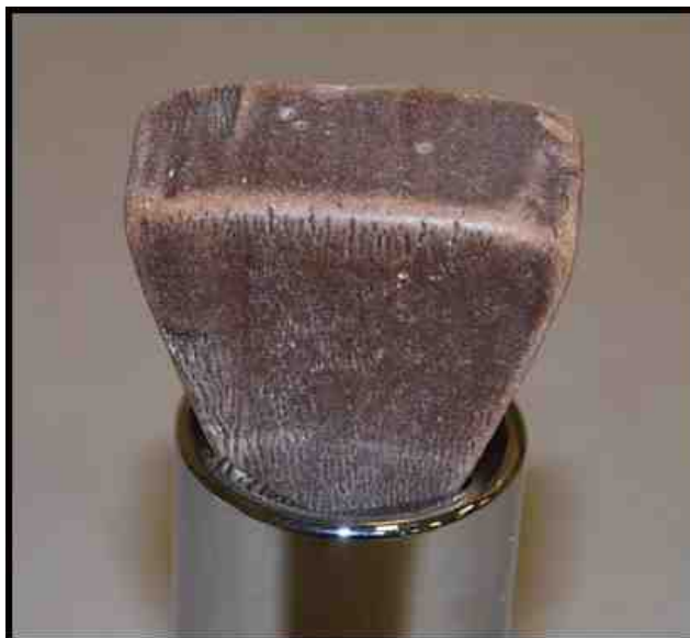
Figure 11 - The same cylindrical part as shown in Fig. 10, except the media size and shape has been changed. Note how the wider base of this isosceles triangle-shaped media prevents it from lodging in the I.D. of the cylinder.
