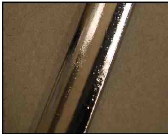
Figure 18 - A plated part showing part-on-part damage - the result of low media level in a vibe bowl.
