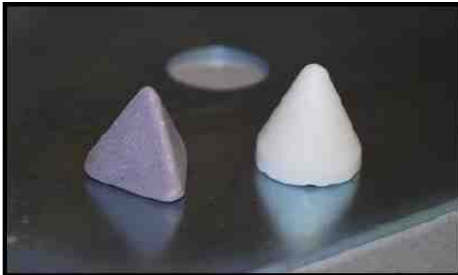
Figure 5 - Additional examples of planar contact patterns. Note that although the cone on the right has curved sides, it demonstrates planar contact when its flat base contacts the flat work piece.
