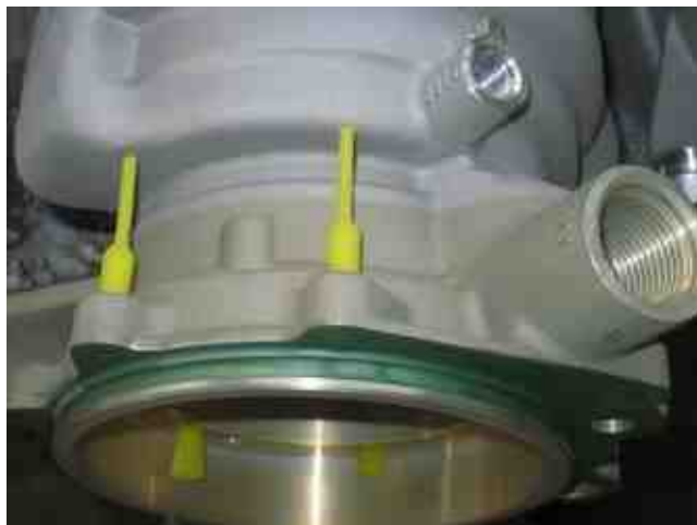
Figure 3 - Masking of holes and protrusions with stoppers and tubing.
