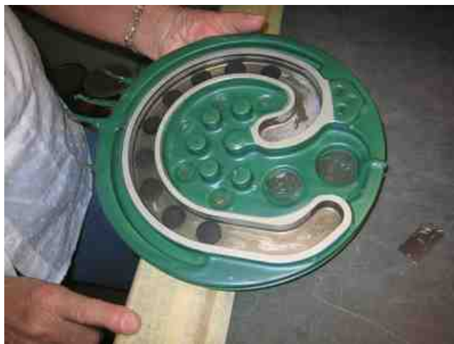
Figure 2 - Example of a polymer/resin-based mask material.
