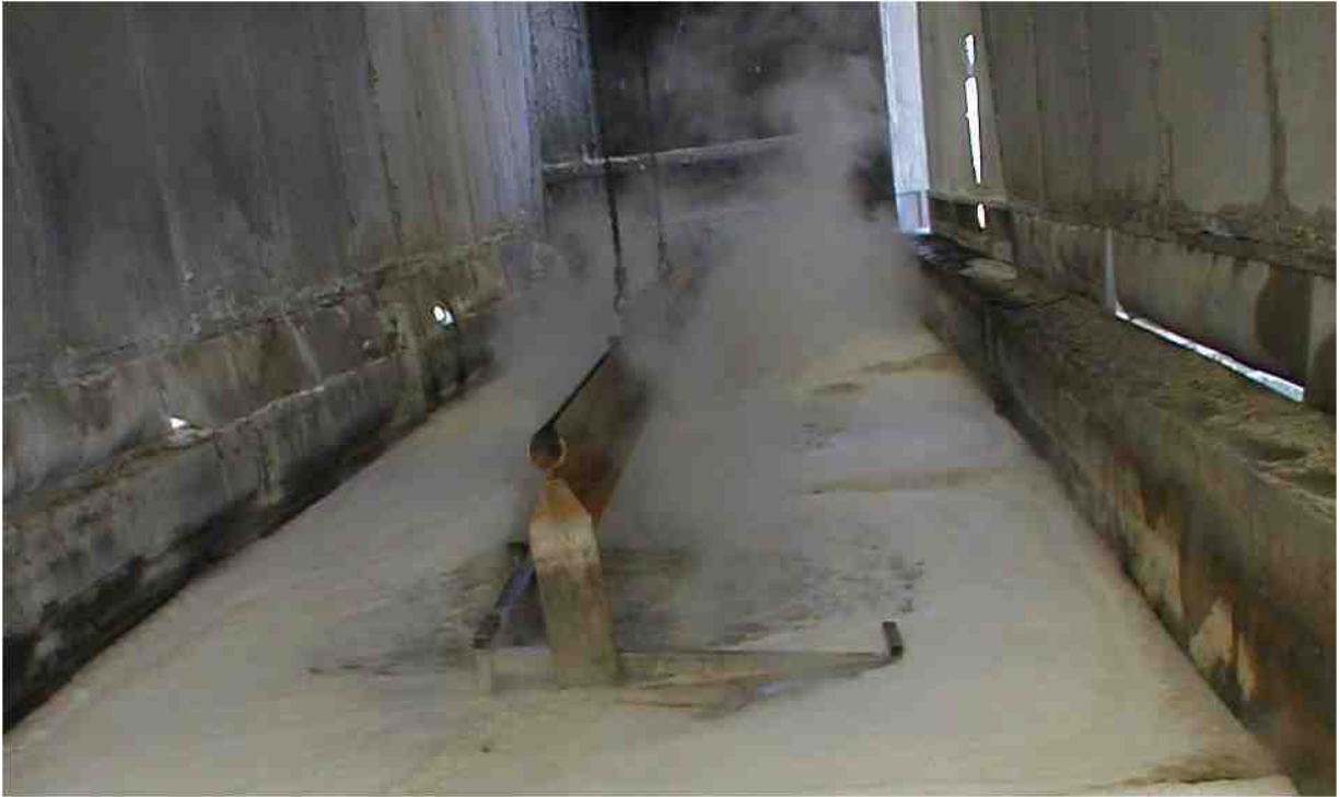
Figure 2 - The part is submerged into the chemical milling etchant.
