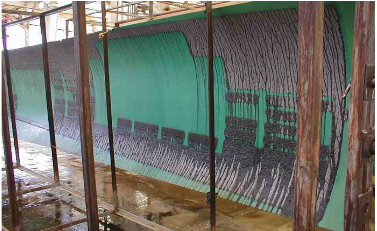
Figure 3 - Appearance immediately after the chemical milling process.
