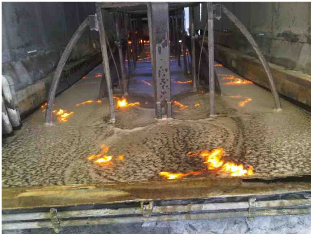
Figure 6 - Hydrogen gas being burned off during the chemical milling process.
