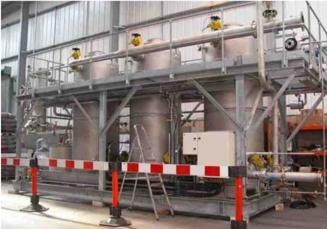
Figure 5 - Three carbon bed adsorber.
