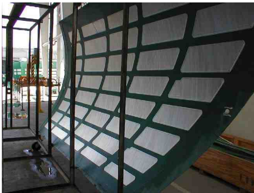
Figure 1 - Sheet aluminum stock is stretched formed and coated with maskant. Select areas of maskant have been removed and the part is ready for the chemical milling process.
